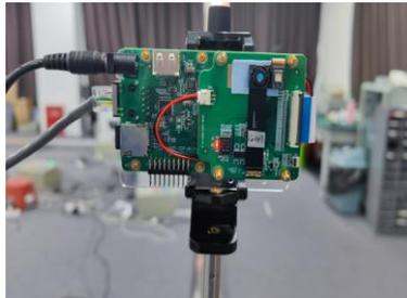
Fig. 8: NV08 area scan TOF camera
