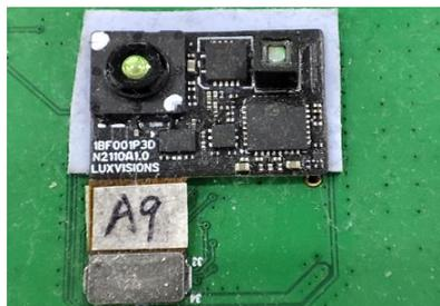
Fig. 9: Installation of the point projection module
